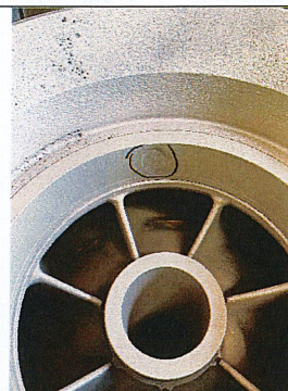
Depression from what appears to have been debris going through the Pump
