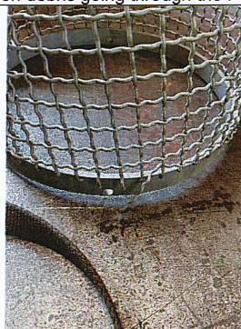
Strainer, ok for reuse after repairs to broken welds
