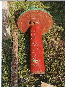
Surface plate and drop pipe – Torch cut due to length
